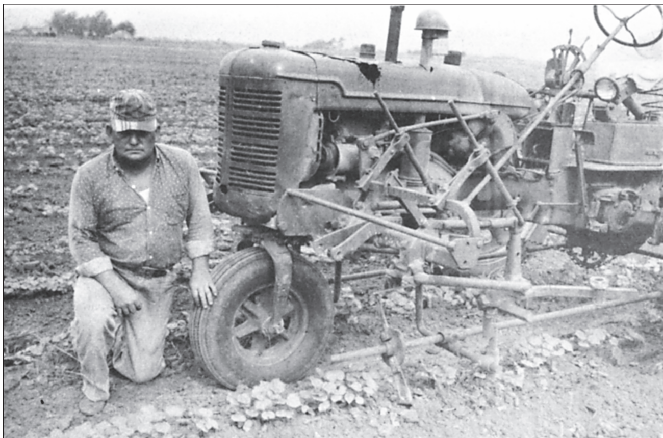
Louis Hohn with mechanical cotton chopper. Hohn produced his cotton with little hand labor on his Eastgate farm.
