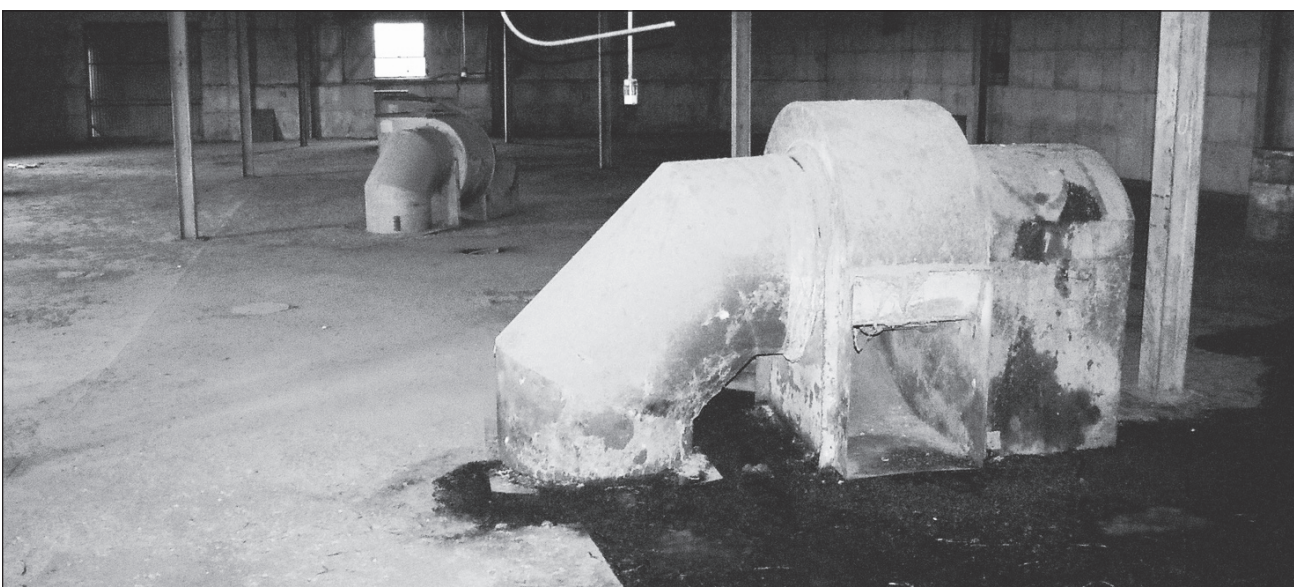
These aerators kept the rice cool so that its temperature didn't rise from naturally-occurring respiration, risking decay.
